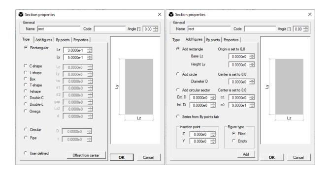
MARNING: it is strongly advised to insert units consistent with the initial choices (see *Edit > Set units*). In the Properties mask it is possible to specify the design properties of the section to be used during checking.
