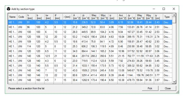
To see the properties (area and moments of inertia) of the inserted sections select a section and press the *Edit properties* button. This mask allows also to import a section from DXF file and define a section by points or by composing single figures.
