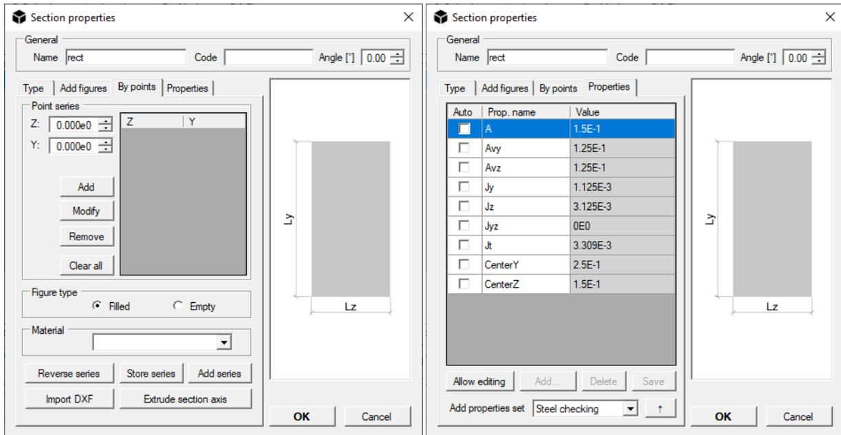
**⚠ WARNING:** by changing the sectional properties, the section will be converted in "Custom" type. Such operation is not reversible.
