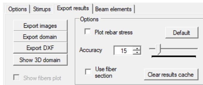
*Beam elements* allows the import of reinforcements from individual elements, temporarily overwriting those of the section. The *Get forces* button allows the stresses for the desired abscissa taken from the calculated model.
