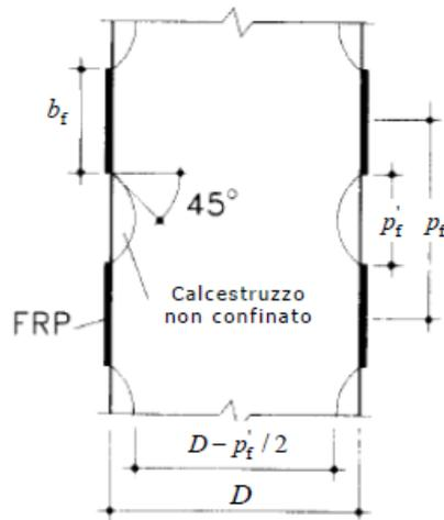
Confinement is only supported for rectangular and circular sections and the radius of curvature  $r_c$  is assumed to be at least 20mm. The effective confining pressure is evaluated as:
