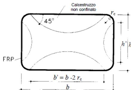
$$\frac{f_{ccd}}{f_{cd}} = 1 + 2.6 \cdot \left( \frac{f_{l,eff}}{f_{cd}} \right)^{2/3}$$
