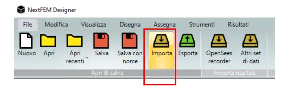
2. Select *Midas GEN text file (\*.mgt)* as the file type from the drop-down list, or drag the MGT/MCT model into the viewport.
